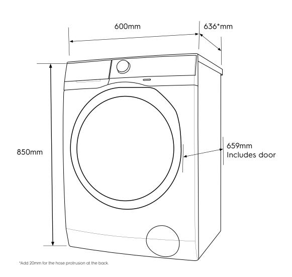
Please note! Dimensions to be used as a guide only. All customers MUST refer to the user manual supplied with the product for detailed installation instructions. © 2021 Electrolux S.E.A PTE. LTD. E\_DIM\_EWW1024P5WB\_Jun21
